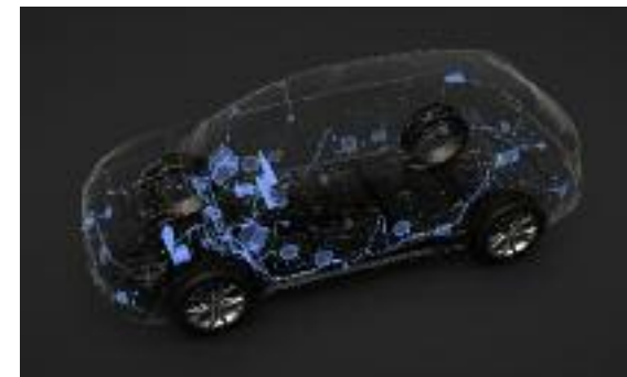
NEA, Groupe PSA's New Electronic Architecture
